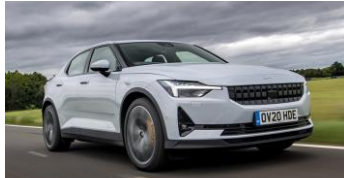
Polestar 2 Type: Pure EV Max power : 300 kW Max Battery : 78 kWh
