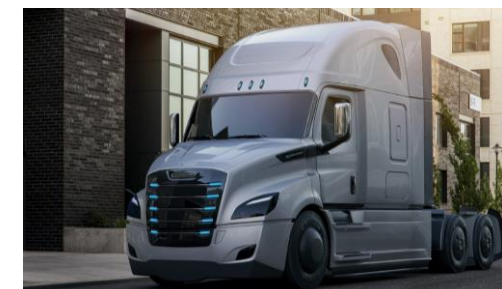
Daimler Freightliner eM2 Type: Pure EV Max range : 370 km Max Battery : 325 kWh
