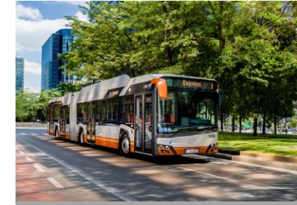
Urbino 12 electric Type: Pure EV Max range : 200 km 7 x battery pack
