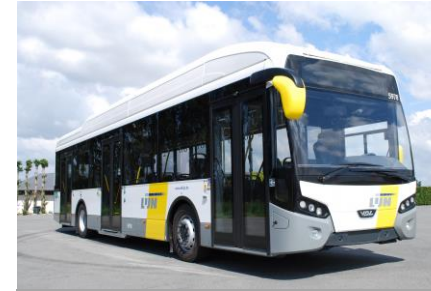
VDL Citea SLF-120 Type: Pure EV Max range : 600 km Max Battery : 216 kWh
