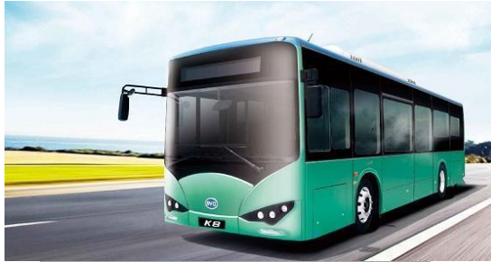
BYD K8 Type: Pure EV Max range : 370 km Max Battery : 250 kWh
